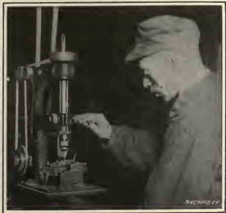
Fig. 167. Drilling Fire-holes in Anvil in a Leland-Gifford High-speed Drilling Machine
