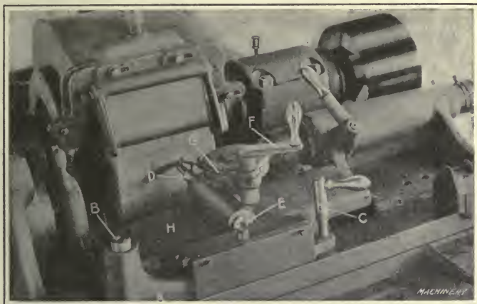
Fig. 121. Wheel-truing Device used on Ford-Smith Grinding Machine
