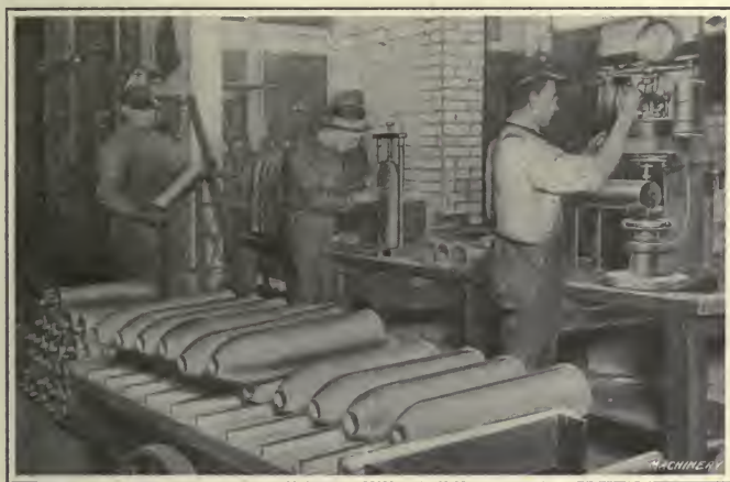
Fig. 81. Testing Hardness of French 120-millimeter High-explosive Shells
