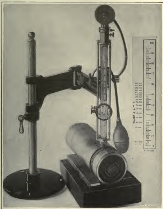
Fig. 117. Testing Hardness of High-explosive Shells with Scleroscope
