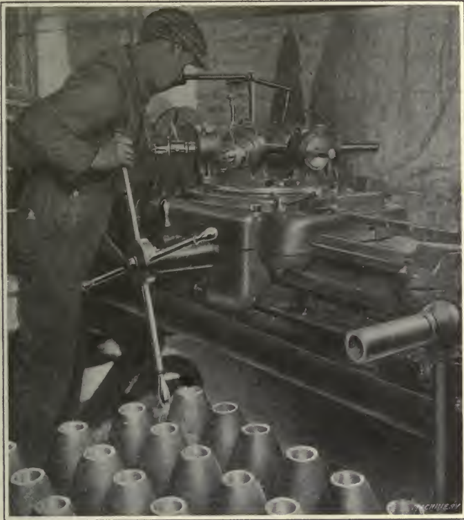
Fig. 83. Boring and threading Open End of Shell on Jones & Lamson Single-spindle Turret Lathe
