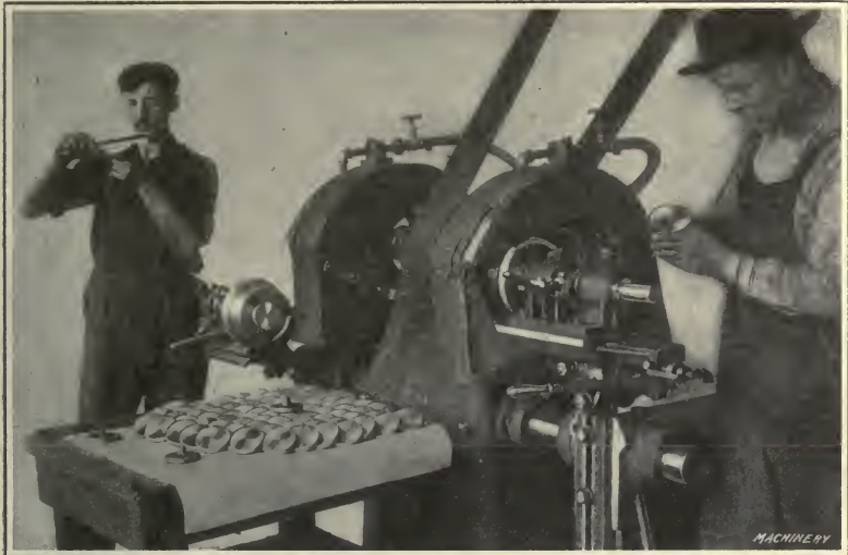
Fig. 114. Surfacing High-explosive Shell Gas Plugs on a Besly No. 14-16-Inch L "Wet" Ring-wheel Grinder
