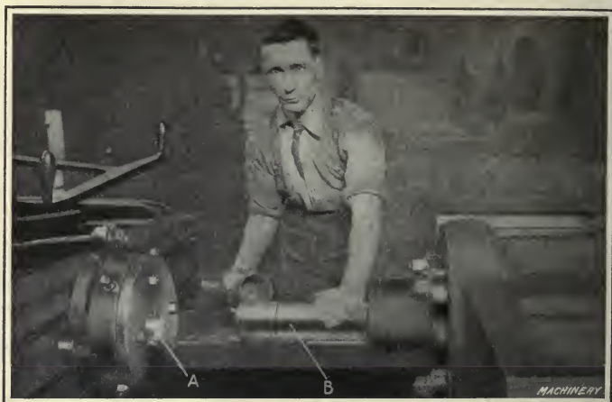
Fig. 172. Third Redrawing Operation on Williams & White Bulldozer
