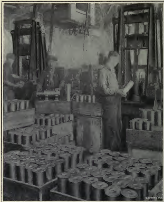
Fig. 153. First and Second Tapering Operations on Special "Toledo" Cartridge Case Tapering Machines
