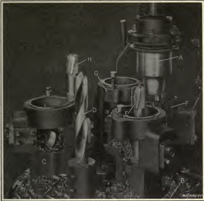
Fig. 42. Close View of Fixture shown in Fig. 41, illustrating Method of applying Tools to Work in an Inverted Position
