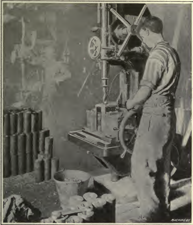
Fig. 28. Baker High-power Drilling Machine at Work on British 18-pound High-explosive Shells
