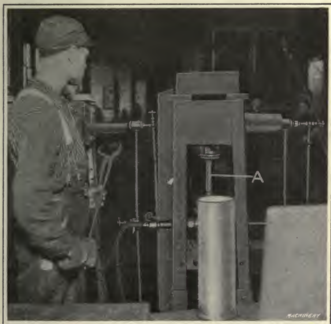
Fig. 175. Mouth-annealing Cartridge Case In an Improvised Annealing Furnace
