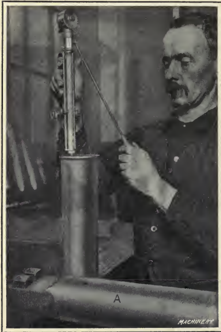
Fig. 179. Testing Hardness of Cartridge Cases with Scleroscope
