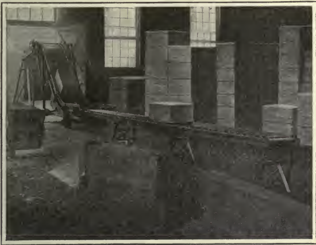
Fig. 124. Mathews Gravity Carrier with Elevator Unit loading Freight Car
