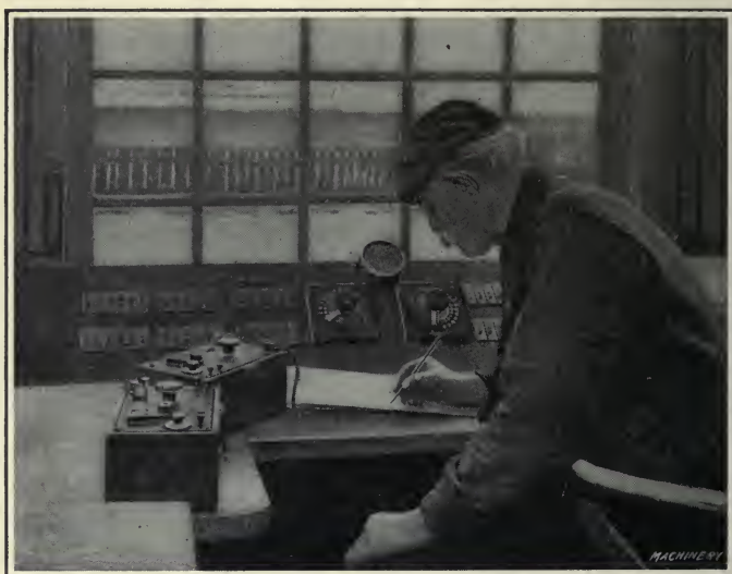
Fig. 142. Recording Instruments used In checking up Temperature of Annealing Furnaces
