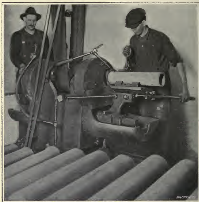
Fig. 68. Grinding Base End of French 120-millimeter High-explosive Shell Forgings in a Gardner Disk Grinder
