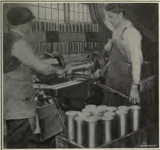
Fig. 150. Trimming Mouth End of Case on a Toledo Cartridge Case Trimming Machine
