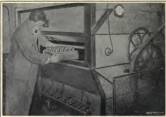
Fig. 137. Baking Varnish on High-explosive Shell Fuses
