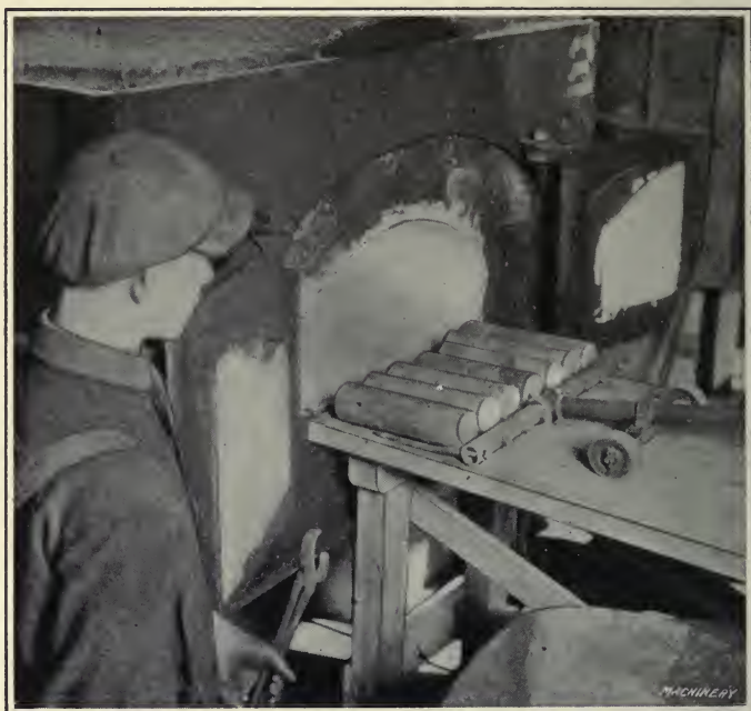
Fig. 50. Heating Russian High-explosive Shell Forgings for Hardening
