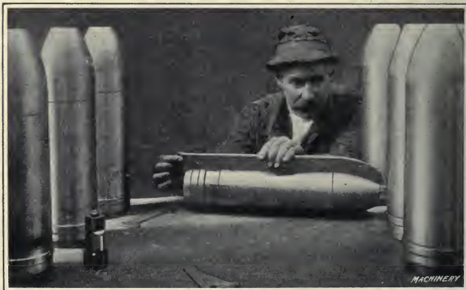
Fig. 90. Gaging Contour of French 120-millimeter High-explosive Shell
