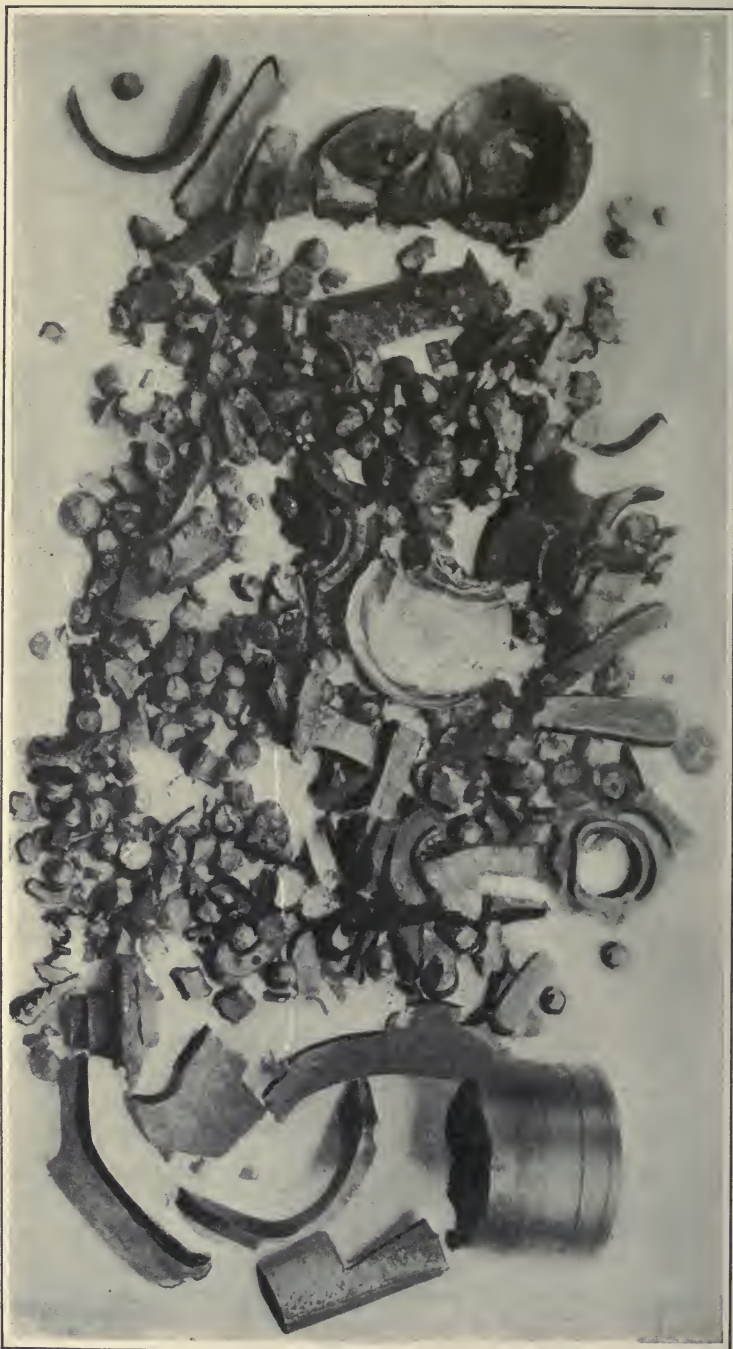
Fig. 4. Condition of an American 3-inch High-explosive Shrapnel after being exploded upon Impact. (Annual Report, Smithsonian Institute, 1914)
