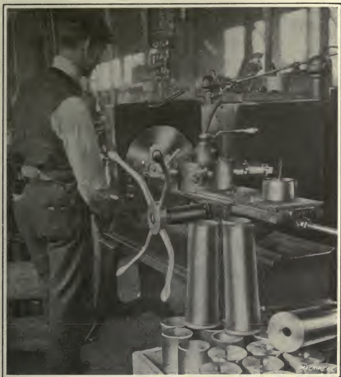
Fig. 154. Machining Head and Mouth Ends of Case on a Bullard Cartridge Case Trimming, Facing and Chamfering Machine
