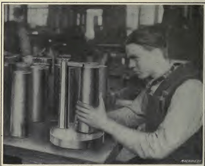
Fig. 158. Gaging Over-all Length of Case
