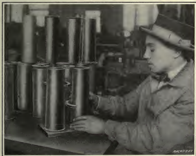
Fig. 157. Testing Taper of Cartridge Case with Horseshoe Gages
